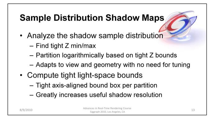
Sample distribution shadow maps address both of these issues by analyzing the actual distribution of light space samples required to shadow the current view.
