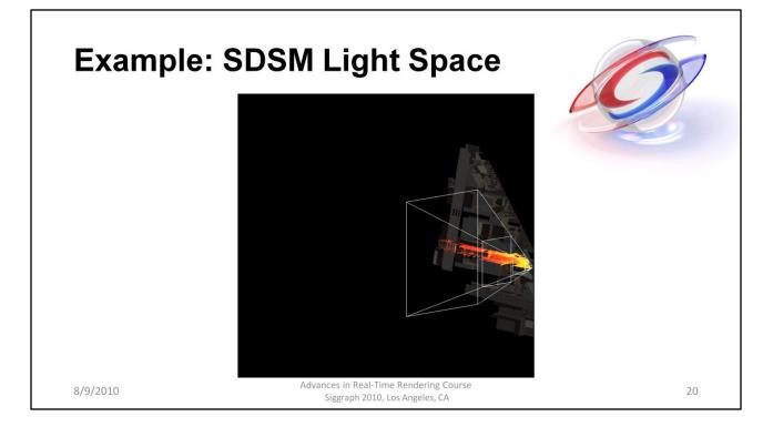
Near/far has been tightened to cover only visible samples. Note that near being tightened is actually the most important.
