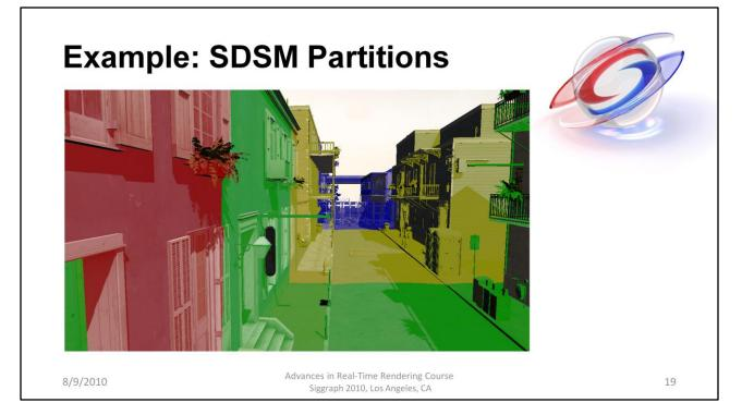
Partitioning is similar to the hand-tuned solution but fully automatic and adapts to the view.
