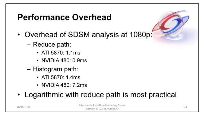
We measured the cost of the SDSM analysis step compared to using static partitions. At 1080p the overhead of the reduce path is around 1ms for these GPUs.
