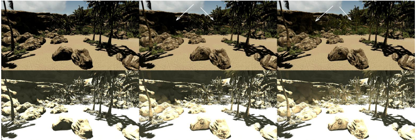
Figure 14. Combination with SSGI. From left to right: pure direct lighting with constant ambient term, light propagation volumes without SSGI, light propagation volumes with SSGI. Diffuse lighting accumulation buffer is shown at the bottom respectively.
