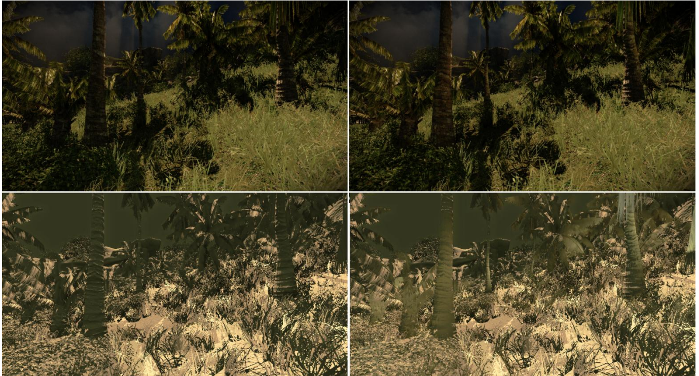
Figure 16. Results of global illumination on consoles (XBox 360 and PlayStation 3). Left: constant ambient term, right: global illumination enabled. Diffuse light accumulation buffer is on the bottom.
