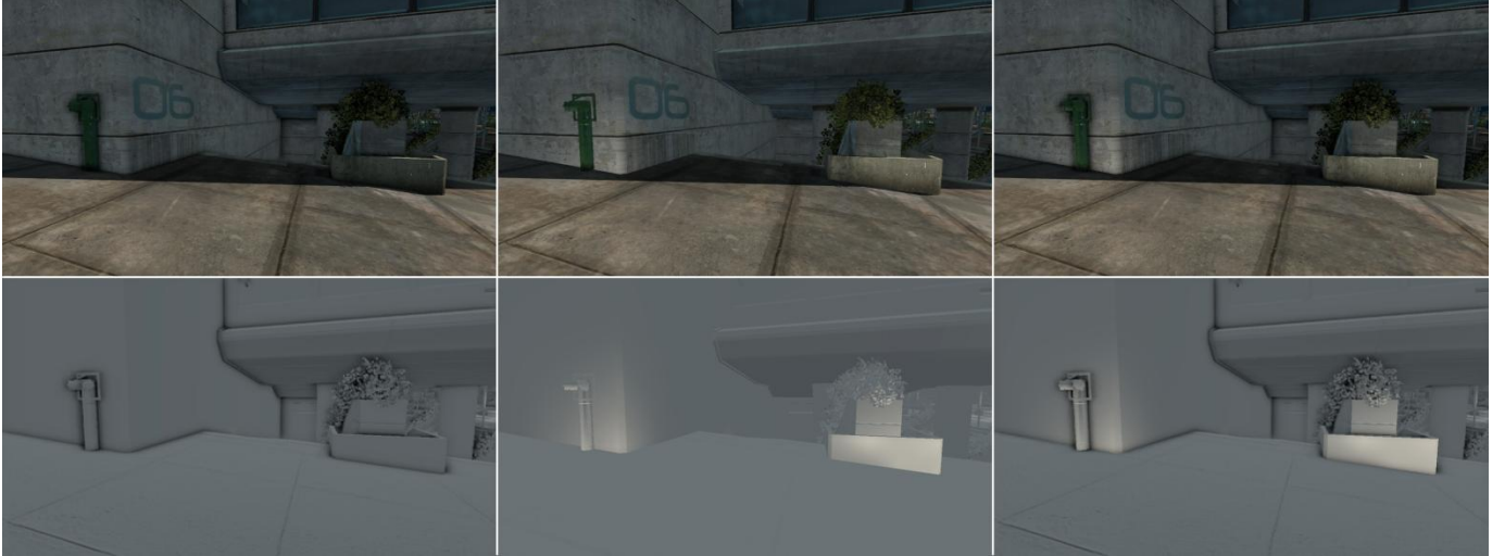
Figure 13. Combination of SSAO and our technique. Left to right: only SSAO, only global illumination, combined approach. The bottom line shows indirect lighting buffer.
