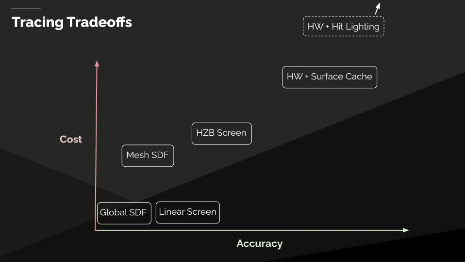
If we graph them all by cost and accuracy, we can see that the Global Distance Field tracing is the fastest, but also the least accurate, and it needs to be complemented with a more accurate method, like the screen traces, or Mesh Distance Field tracing.
