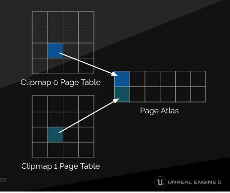
The global distance field merges all mesh distance fields and heightfields into a set of clipmaps centered around the camera. Mesh distance fields and heightfields are a perfect mesh representation for this as they are simple to merge and LOD at runtime.
