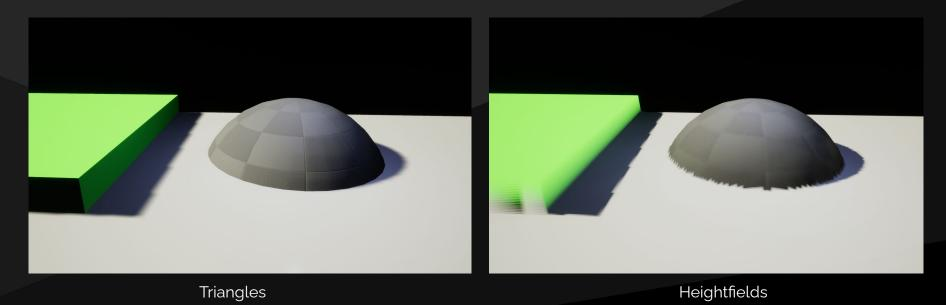
When we started working on Software Ray Tracing, one of the first things we tried was to capture the scene using a bunch of orthographic cameras, giving what we call cards. We then ray trace through the card heightfields, and sample the card lighting when the ray hits.
