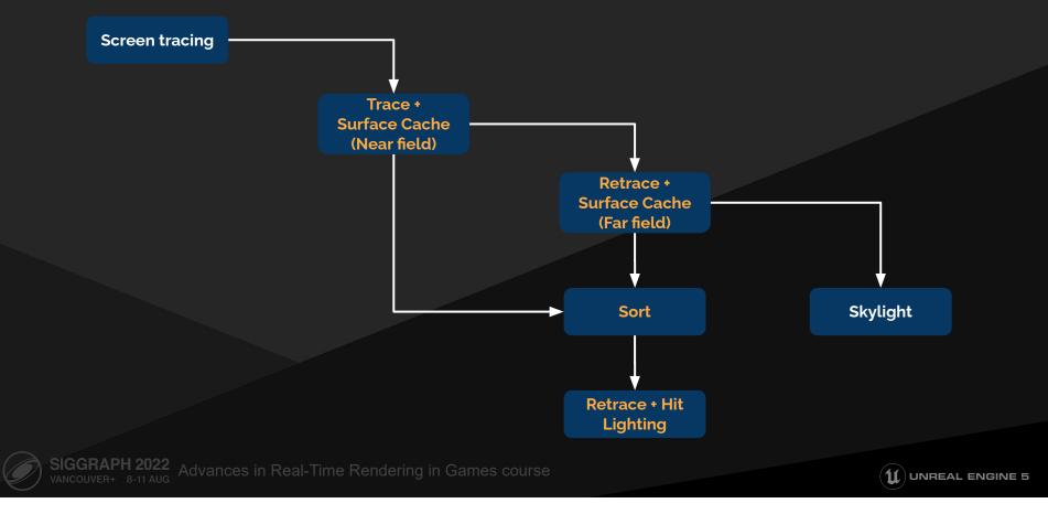
With some reordering of stages, we can minimize the dispatch costs by first resolving all Surface-Cache stages before optionally requeuing results for Hit-Lighting. We do this by cascading through both geometric representations. Hits are then compacted and optionally requeued for Hit-Lighting, while misses cascade to apply SkyLight evaluation.
