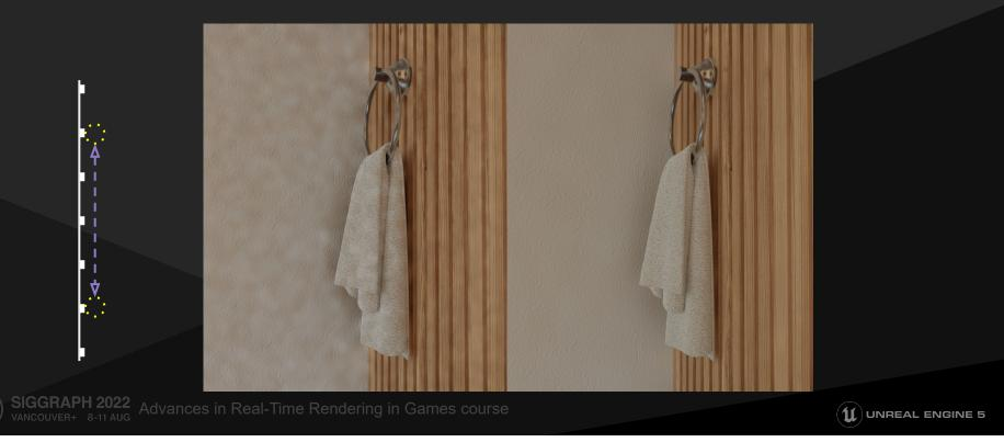
It provides large spatial filters for cheap, because we're filtering in the Radiance Cache space and not in screen space. A very small 3x3 filtering kernel in the probe space gives us the same noise reduction that a large 48x48 screen space filtering kernel would do. We only have to load the positions of the probes, rather than all the positions and normals of all the pixels for error weighting.
