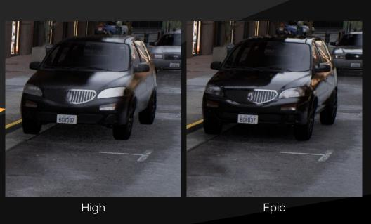
In "The Matrix Awakens", we're using Hardware Ray Tracing with Far Field, and it's a much more complex scene so our tracing costs are higher. On High settings the total Lumen cost is 6.4 milliseconds, while Epic has significantly higher quality at 11.3 milliseconds.
