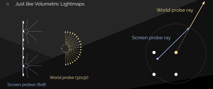
The World Space Radiance Cache is handling distant lighting, with higher directional resolution but lower spatial resolution. It solves the problem where all of the lighting in a room is coming from a small distant window, which was missed with a small number of rays. We integrate the two radiance caches by shortening the Screen probe ray, and when it misses we interpolate from the World Space Radiance Cache.
