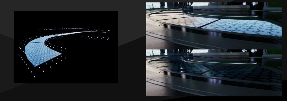
For the rest of the layers, we use the World Space Radiance Cache again. We use the same Radiance Cache as the Opaque Final Gather, we just need to place some more probes. We mark the new probes by rasterizing the translucent surfaces at a low resolution, and then mark the probes that are needed at each pixel's position.
