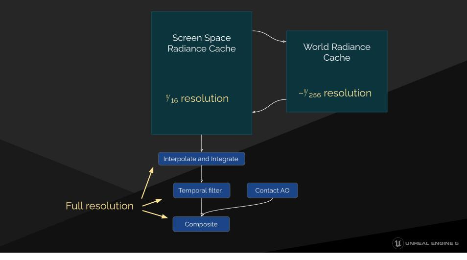
The opaque Final Gather has three main parts, first there's the Screen Space Radiance Cache which is operating at 1/16th resolution in each dimension. It's backed up by the World Space Radiance Cache, which is handling distant lighting at a much lower resolution. At full resolution there's the interpolation, integration, the temporal filter and Contact AO.
