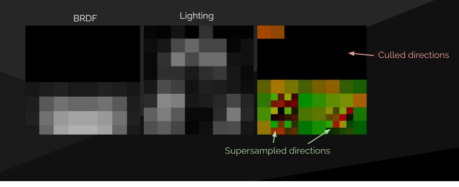
We're operating in a downsampled space, so we can afford to launch a whole threadgroup per probe to do better sampling. Product Importance Sampling is normally only possible in offline rendering, but we can do it in real-time.
