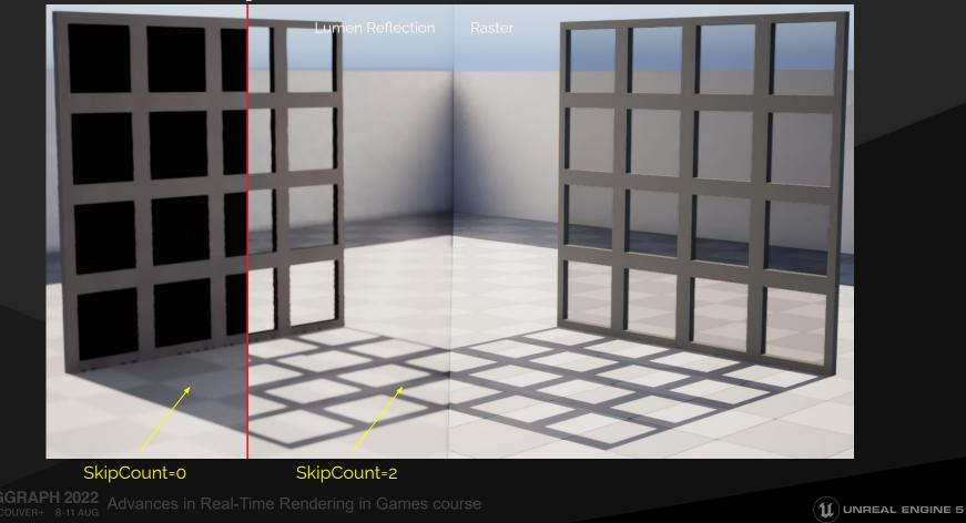
This example shows the application of MaxTranslucentSkipCount when encountering a translucent geometry segment.
