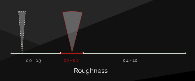
We can solve the incoherency in the roughest reflections by just reusing the work that we did for Diffuse GI. The Screen Space Radiance Cache has enough directional resolution for a wide specular lobe, and we can just resample it, by importance sampling the GGX lobe to get a direction, and then interpolating radiance from the screen probes.
