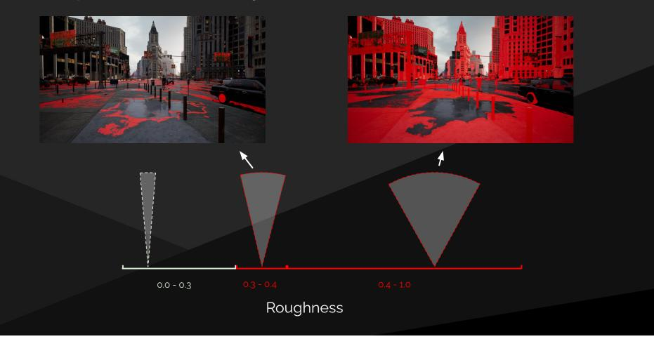
One of the problems we have with reflections is the slow tracing of incoherent rays. When the material's roughness approaches 1, the GGX lobe approaches diffuse and our rays become very incoherent.
