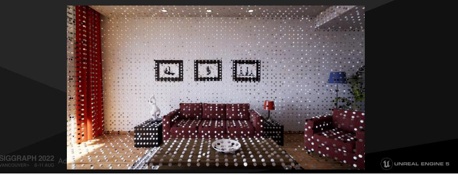
Ideally we would trace at least 64 rays from every texel, but that's just too expensive. Instead we place a hemispherical probe on 4x4 tile and trace only from probe texels. This enables downsampled tracing and still preserves surface normal detail.
