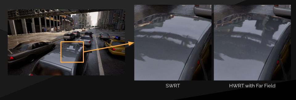
In 'The Matrix Awakens' tech demo, the cost of both tracing methods is nearly the same. Hardware Ray Tracing gives higher quality reflections and supports GI over huge view ranges with Far Field, so it's the better choice.
