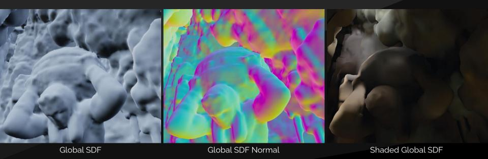
For global distance field tracing we loop over clipmaps starting from the smallest one and raymarch each one of them until we find a hit.
