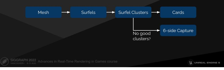
In order to place cards on a mesh we run a precomputation step during mesh import.
