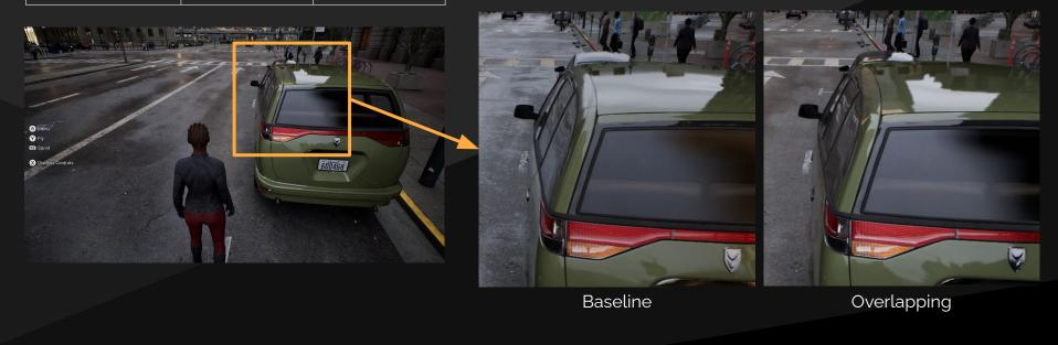
Submitting both near-field and far-field representations to the same top-level acceleration structure is NOT ideal. Doing so creates needless geometric overlap. While the ray-mask removes unnecessary traversal, the damage to the top-level acceleration structure build is substantial. Our early experiments with overlaying the far-field representation revealed a show-stopping 44% penalty to all near-field traversal costs.
