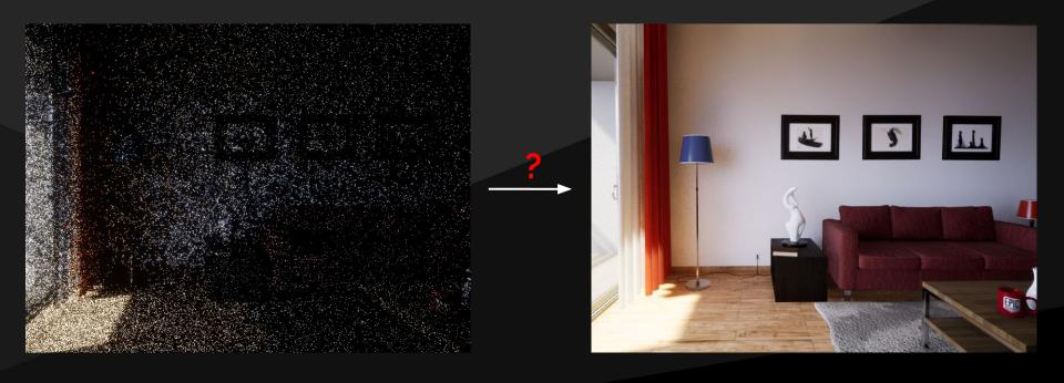
The third fundamental problem that we have to solve for realtime global illumination is the noise in the light transfer, considering that we can't even afford one ray per pixel for diffuse GI, but we actually need hundreds of effective samples for high quality indoors.
