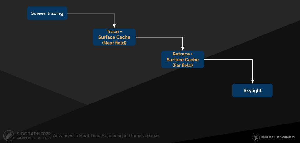
Incorporation of far-field traces into ordered traversal places a new set of stages into our original hardware traversal pipeline. We add an intermediary compaction step, collating near-field misses into new ray-tiles, and then a subsequent indirect dispatch to trace the ray-tiles against the far-field representation.
