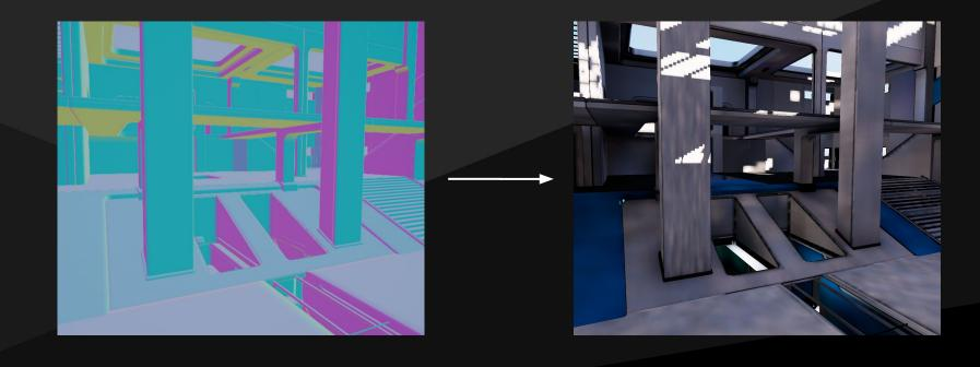
We interpolate the lighting where the ray trace hit from the cards, which we call the Surface Cache. Areas that are missing coverage only result in lost energy, instead of leaking. Ray tracing the card heightfields didn't work, but using them for lighting does.
