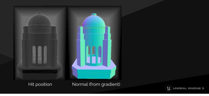
So instead we settled on Mesh Signed Distance Fields for our Software Ray Tracing geometry representation. These give reliable occlusion, all areas have coverage, and we still get fast software ray tracing through sphere tracing, which skips through empty space. The intersection with the distance field surface only gives us the hit position and normal, we can't find the material attributes or the lighting.
