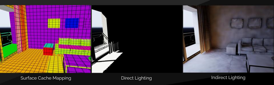
Surface cache contains all mesh and material data and we can use it to evaluate and cache lighting.
