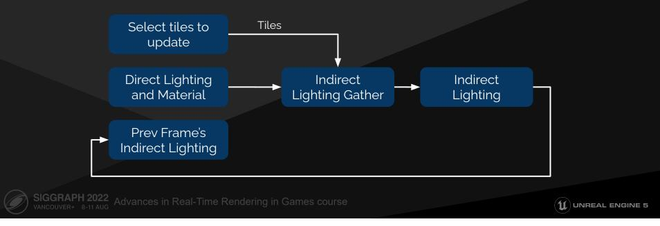
Indirect lighting is more challenging as here we basically need to run the final gather in surface space to compute the secondary bounce.
