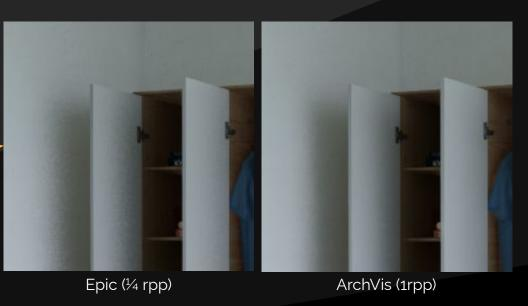
Now looking at an Architectural Visualization scene, running on a 2080 TI. On Epic settings Lumen costs 7.3 milliseconds, which has a little bit of noise visible when you zoom in on one area of the screen. We can crank up the Final Gather to 1 ray per pixel, and now we have extremely smooth indirect lighting.
