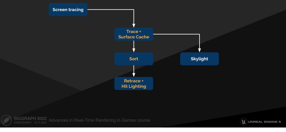
This allows us to repurpose the Surface-Cache tracing stage as the prerequisite to the Hit-Lighting pipeline. It also grants us the flexibility to optionally invoke dynamic evaluation on a per-ray basis. For instance, we have experimented with this idea to optionally invoke Hit-Lighting on meshes which have no Surface Cache parameterization.
