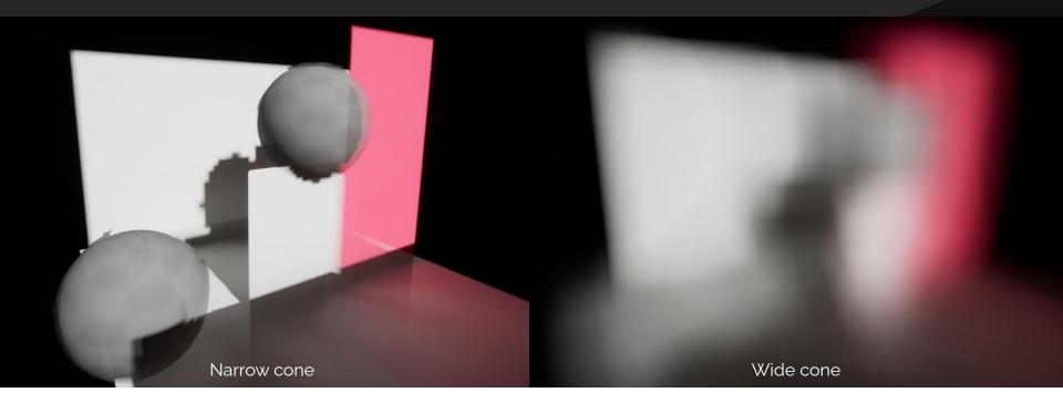
We implemented cone tracing against Mesh Signed Distance Fields. Whenever the cone intersects a surface, we calculate the mip of the surface cache to sample using the size of the cone intersection, giving prefiltered lighting for cones that intersect.
