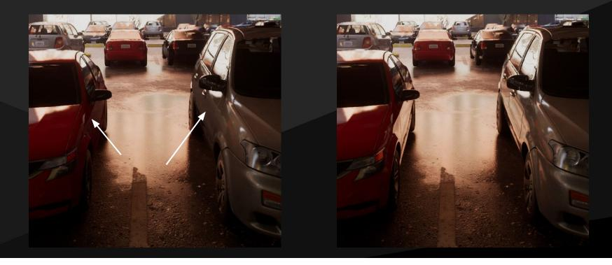
Ultimately, Screen traces are a net quality win, although the more they do, the more you notice when they fail. With Hardware Ray Tracing they also give a small performance win as they allow most of the rays to escape the complex surface geometry.
