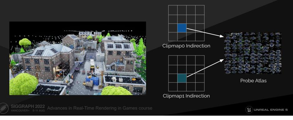
The World Space Radiance Cache has sparse coverage, and we use a clipmap distribution to maintain a bounded screen distance between the probes, to make sure that we don't over-sample, or under-sample.
