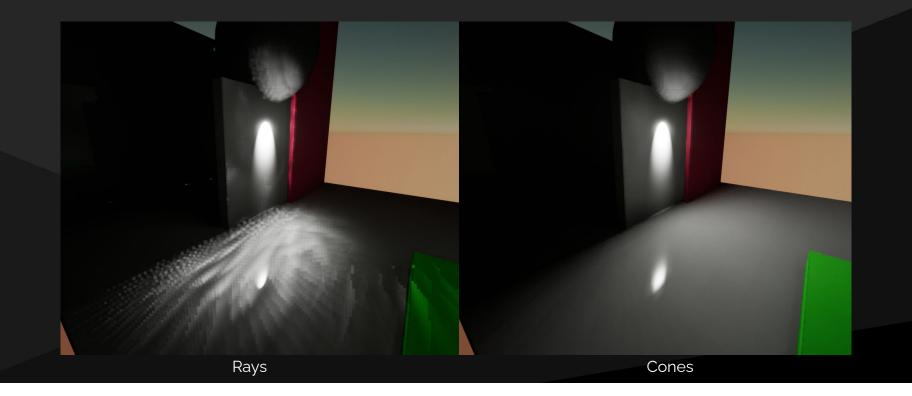
One of our early experiments was prefiltered cone tracing. It's very difficult to implement, but if you can pull it off, tracing a single cone gives you the results of many rays. Cones can be very effective at solving noise and they essentially make the Final Gather trivial.
