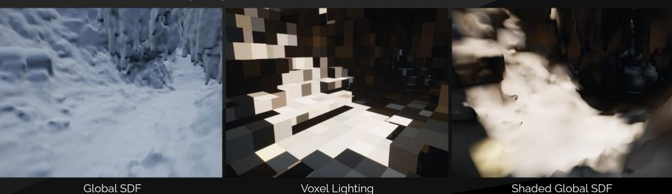
One last issue is that we can't sample surface cache directly from the global distance field traces. Global distance field is a merged scene representation and we don't know which mesh instance was hit.
