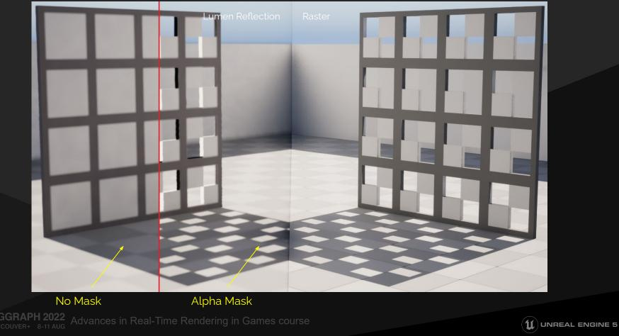
This example shows the application of evaluating surface-cache opacity to reconstruct the geometry's alpha mask during traversal.
