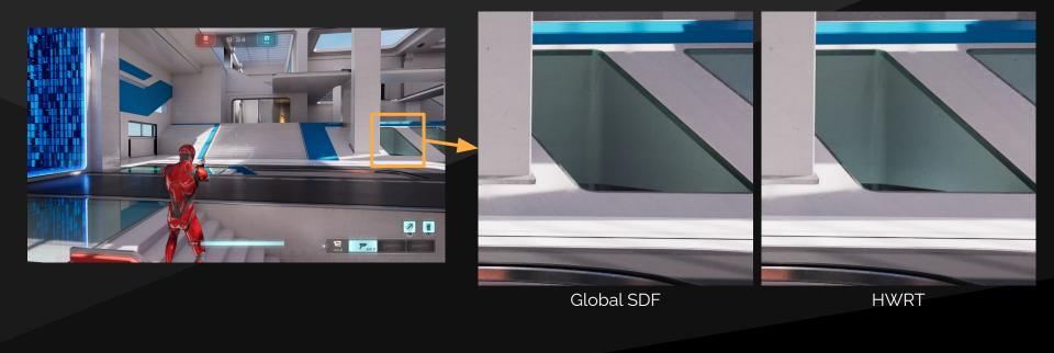
In the Lyra UE5 sample game, it's a different situation. The geometry here is not really overlapping, so Hardware Ray Tracing performs very well. The cost difference between the two techniques is not that large, and neither is the quality difference. It could really go either way, depending on what the hardware supports.
