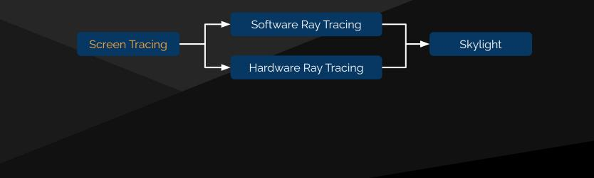
Lumen uses a hybrid ray tracing pipeline, which allows us to mix and match different techniques. Screen tracing goes first, and then each tracing method hands off to the next, by writing out how far the ray traversed, and whether it found a hit or not. The next tracing method can then resume the ray, picking up where the previous method left off.
