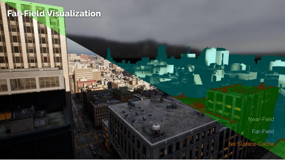
This visualization shows the delineation of near-field and far-field geometry. Geometry which does not have a surface cache entry is also highlighted.
