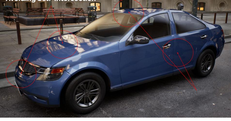
Here is an example of the common self-intersection artifacts we encountered when rendering the vehicles in the demo. I have specifically disabled screen traces to show the prevalence of the artifacts when relying only on the ray-tracing scene.
