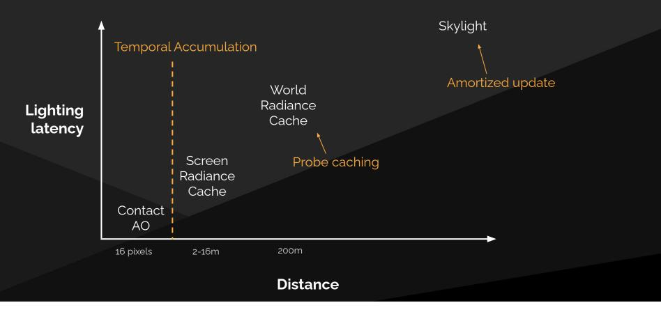
We can take advantage of allowable latency in the Screen Space Radiance Cache by temporally accumulating it, while the World Space Radiance Cache can reuse whole probes from previous frames, and the skylight can be slowly updated over many frames.
