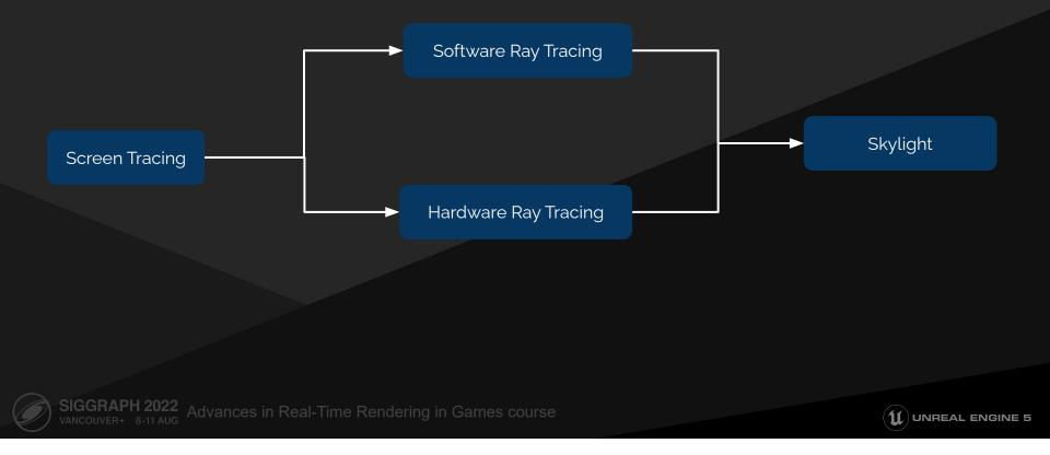
Here's Lumen's ray tracing pipeline, starting from Screen Tracing, which we run first, because it's the most accurate near the start of the ray, then we do Software Ray Tracing or Hardware, depending on what is configured, and finally skylight if the ray misses any geometry.
